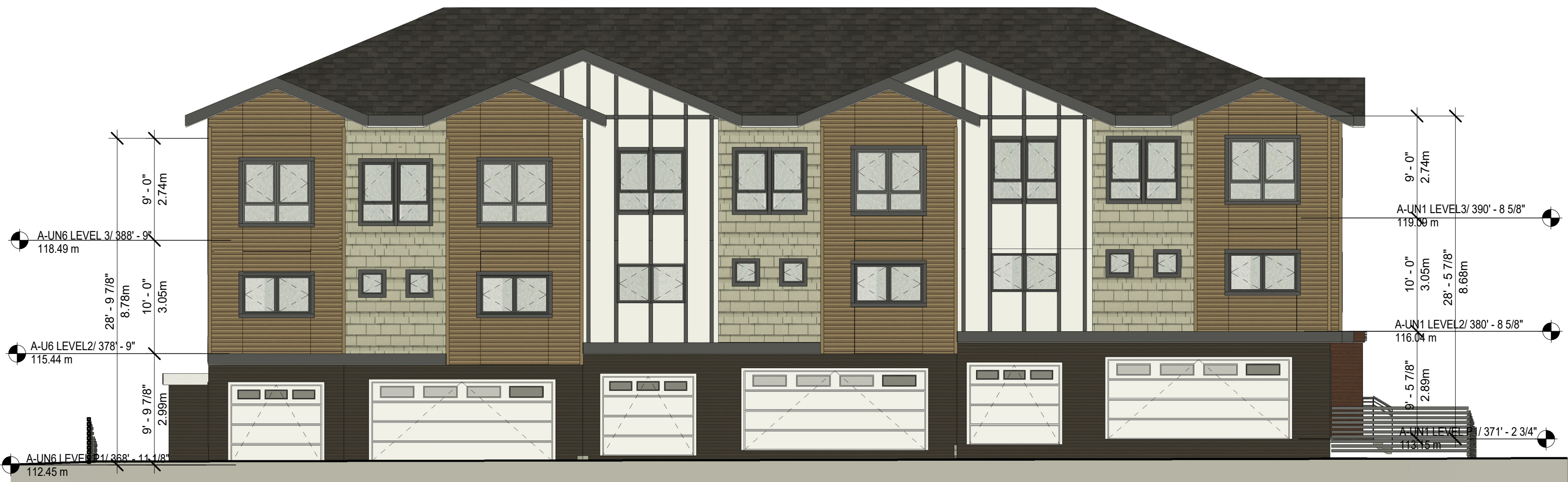
② Elevation BLD A - South (Driveway) 1/8" = 1'-0"
