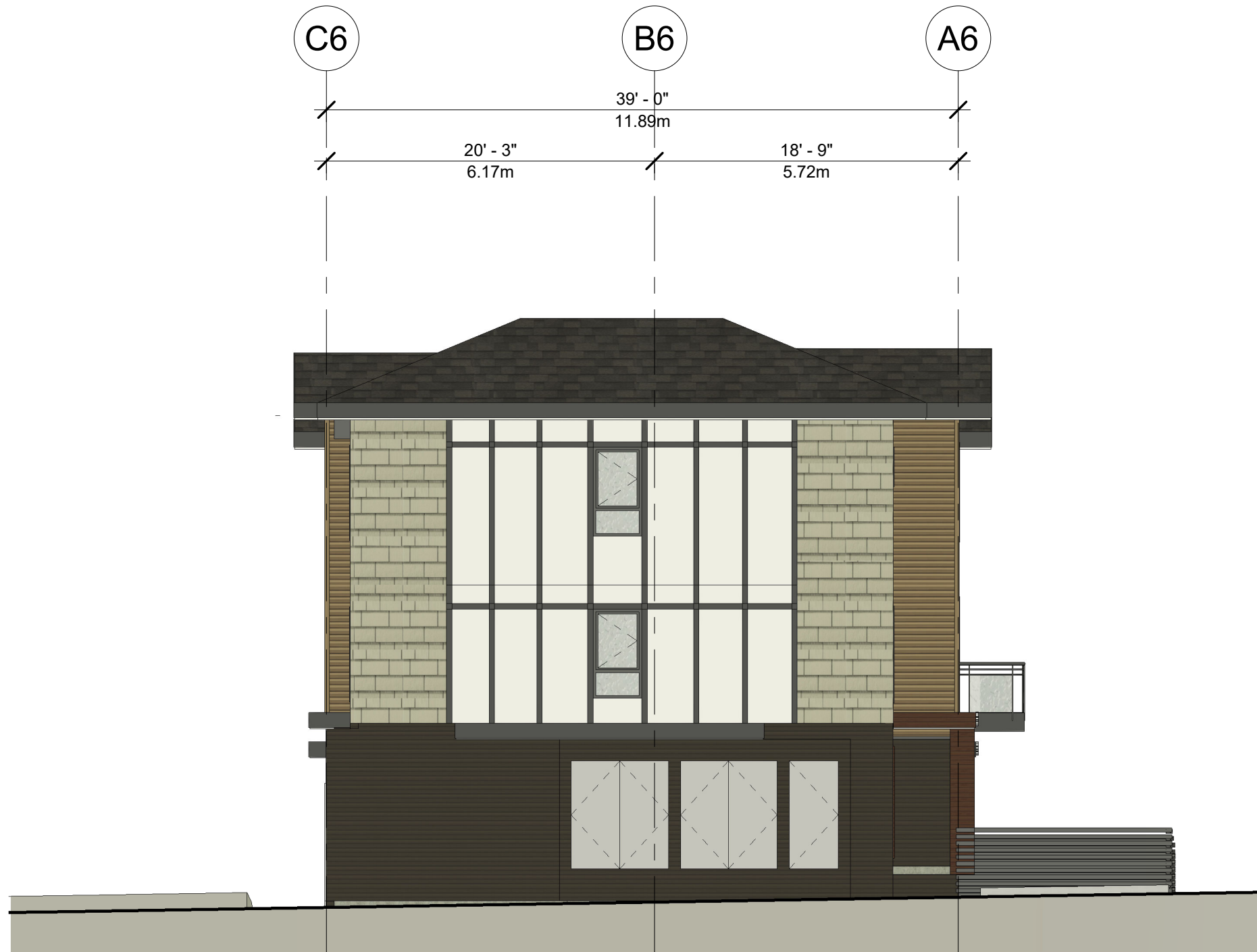
④ Elevation BLD F - South (Left Side) 1/8" = 1'-0"
