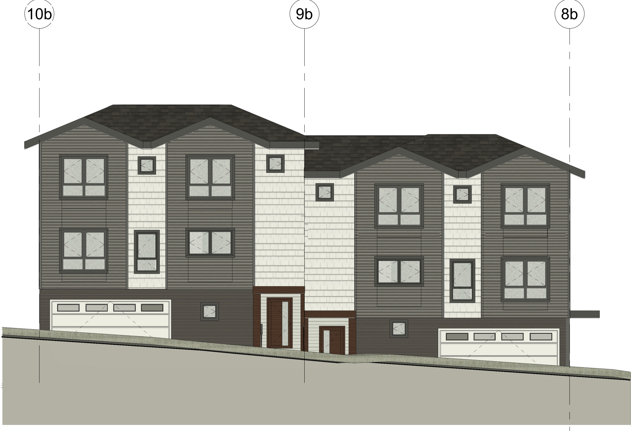
③ Elevation BLD B - East 1/8" = 1'-0"
